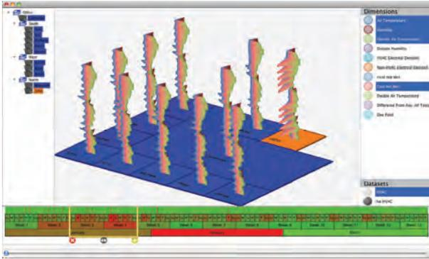
**Figure 4. Prototype system overview. From each sensor location in this floor plan, a Wakame grows vertically over time. The profile at every height is derived from the multi-dimensional data collected at that moment. Controls around the border allow for the specification of time ranges as well as the constraining of displayed dimensions and Wakame.**
